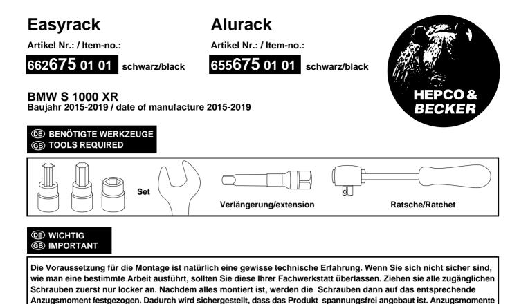
Of course, the assembly requires a certain technical experience. If you are not sure how to execute a determined action, you should ask your local distributor to do it. First, tighten all screws only loosely. After mounting all parts, the screws should be tightened to the torque specified. This guarantees, that the product is mounted without tension. Observe the tightening torques of the manufacturer! Control all screw connections after the assembling for tightness!
